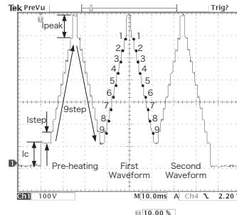
[C terminal voltage waveform connected resistor as D.U.T]
